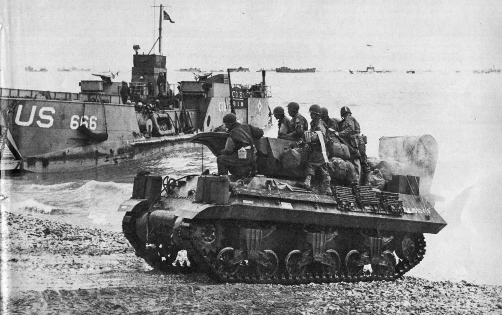
M-10 TANK DESTROYER CLIMBS NORMANDY BEACH WITH GUN REVERSED. PAIRED BOGIE WHEELS, FRONT DRIVING SPROCKET TYPIFY U. S. DESIGN
